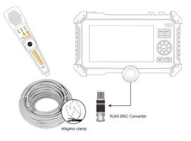
**Locate cables**: Arrow keys to switch mode, "UTP mode" to looking for unshielded network or telephone cables, "BNC mode" for finding BNC cable after connecting adapter. "STP mode" is used to find the shielded network cable. Turn on the cable tracer. The round knob, if clockwise rotation the knob to increase sensitivity, and turn it counter clockwise to decrease the sensitivity.
